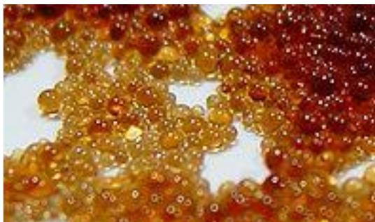
**Fig.1.2.7. Limescale in a PVC pipe. Fig. 1.2.8. Ion exchange resin in the form of beads.**
