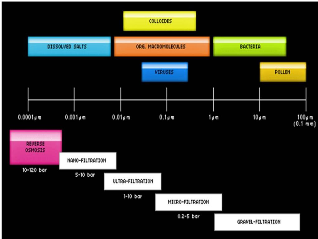
Fig.1.3.11. Depending on the type of membrane used various pollutants incl. microplasts can be removed from water.
