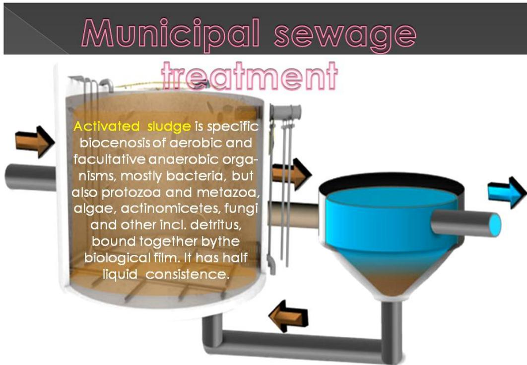
**Fig. 1.3.4.** Sketch of secondary sewage treatment in activated sludge tank connected with secondary clarifier (activation – intensification of processes ongoing in nature).
