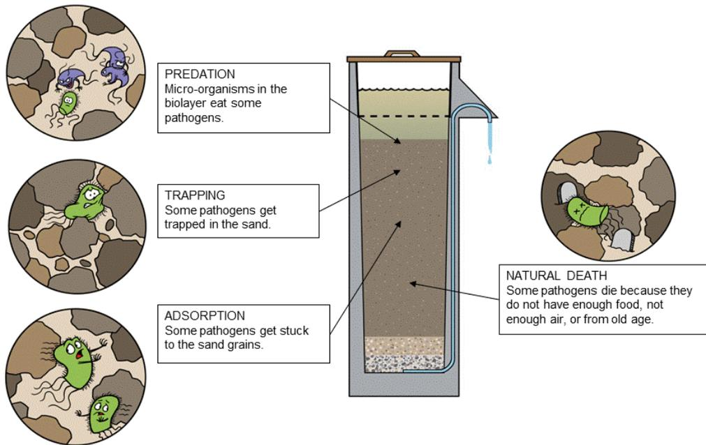
**Fig. 1.2.2. Principle of mechanical sand filtration.**
