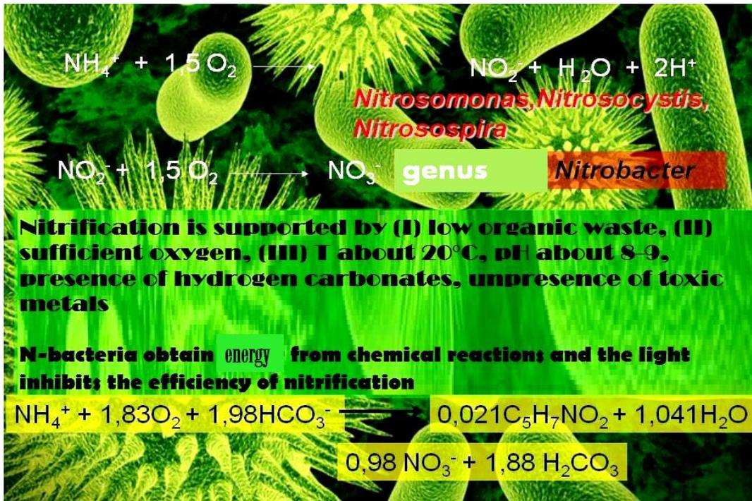
Fig. 1.3.6. Layout of nitrification process by chemical equations.
