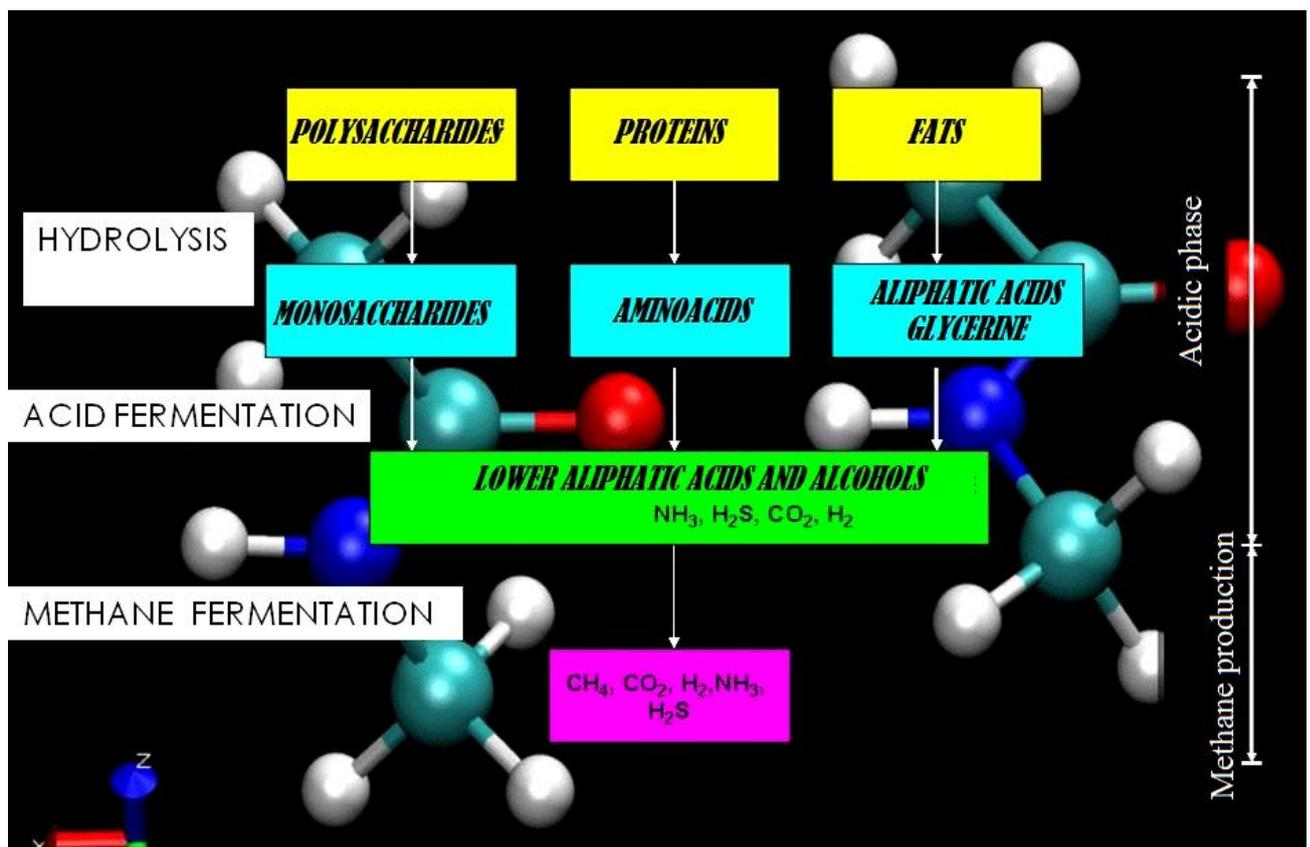
Fig. 1.3.14. Biochemical process layout for the anaerobic digestion.
