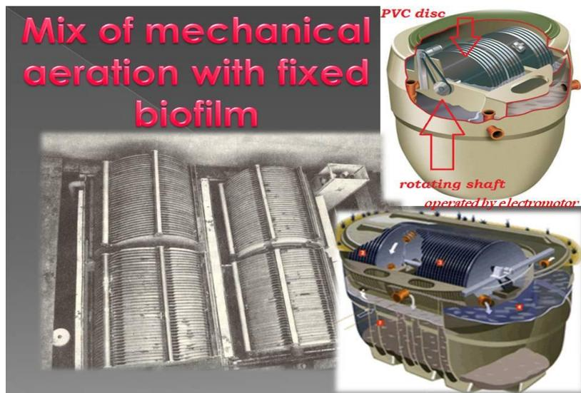
**Fig.1.3.1. Municipal wastewater treatment using biodiscs.**
