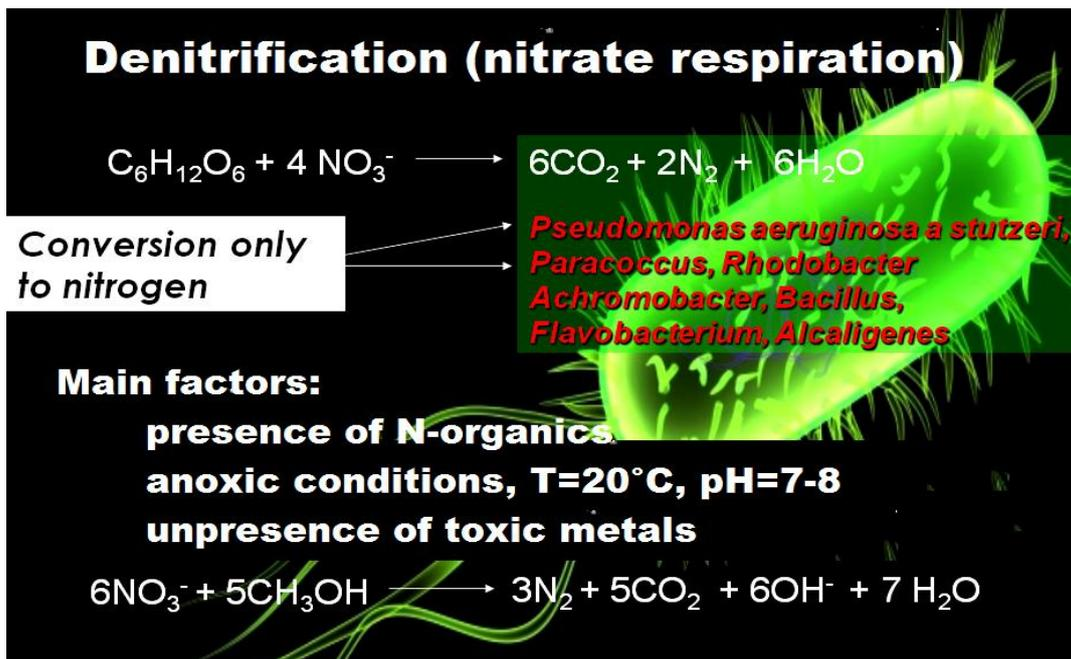
Fig. 1.3.7. Layout of denitrification process by chemical equations.
