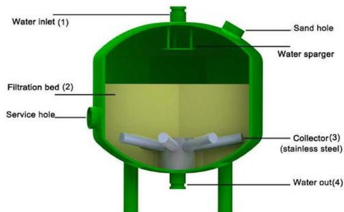
**Fig. 1.2.3. Commercial steel pressure filter composition.**
