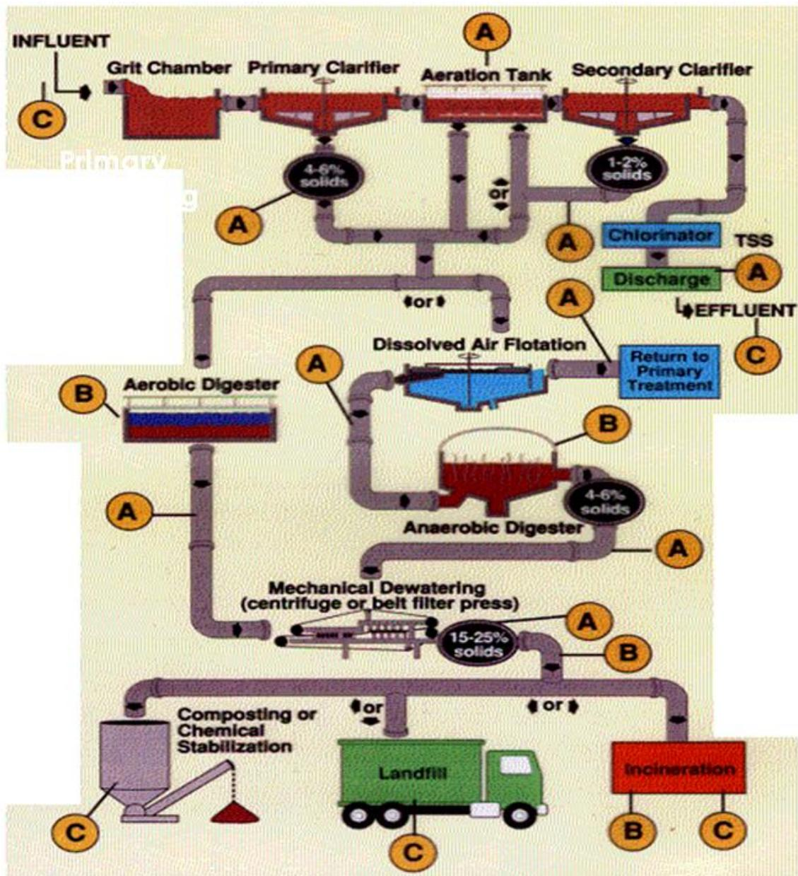
Fig. 1.3.13. Scheme of the entire wastewater treatment plant incl. sludge handling.
