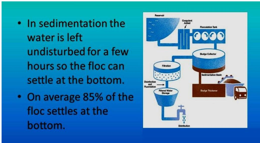
**Fig. 1.2.5. Sketch of surface water purification incl. coagulation and flocculation.**
