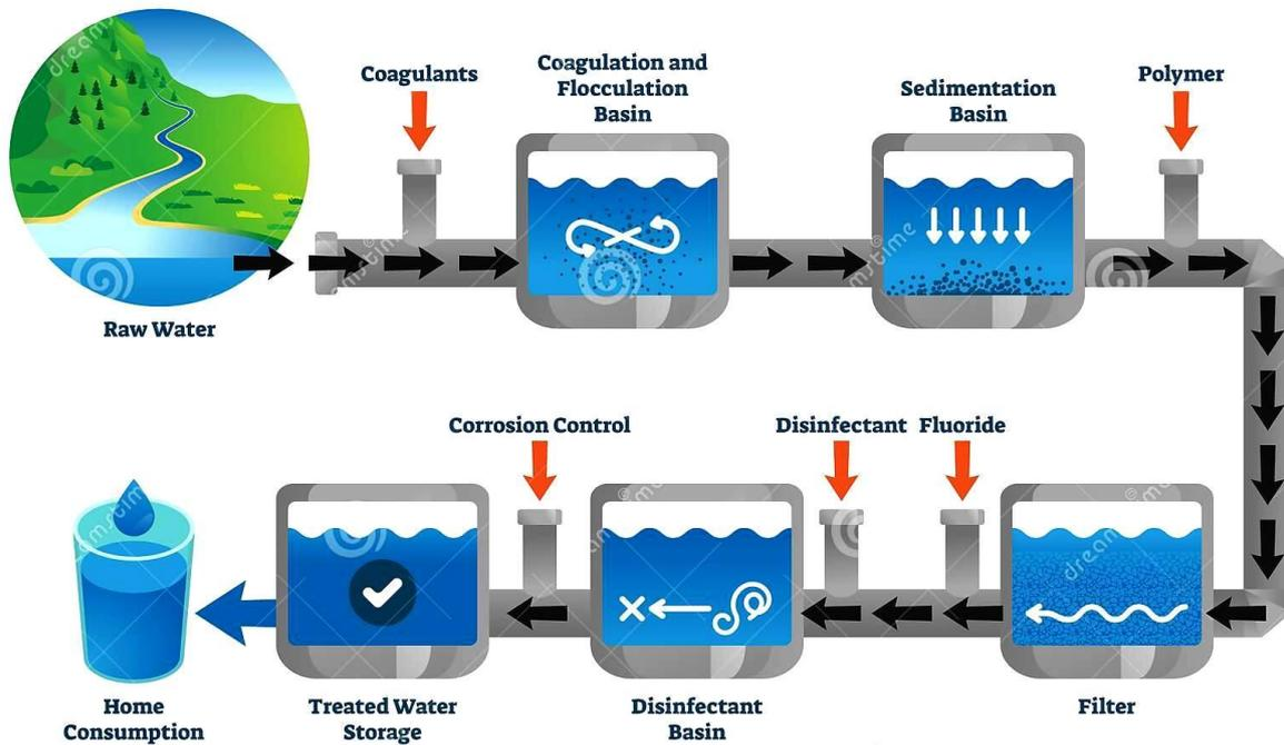
Fig. 1.2.10. Scheme of conventional surface water purification in waterworks (upper figure a typical surface water pumping into waterworks from the middle of reservoir).
