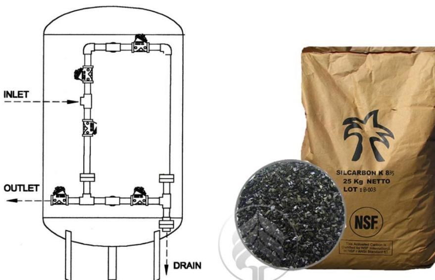
Fig. 1.3.12. Principal sketch of pressure filter (left) which may be filled with activated carbon (right).
