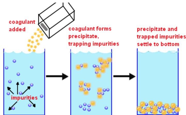
**Fig. 1.2.4. Basic process explanation for coagulation and flocculation.**
