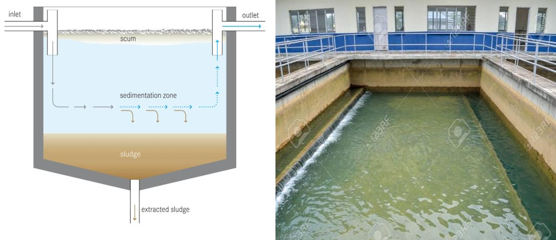
**Fig. 1.2.1. Sketch of sedimentation tank (left) and sedimentation basin in real waterworks (right).**
